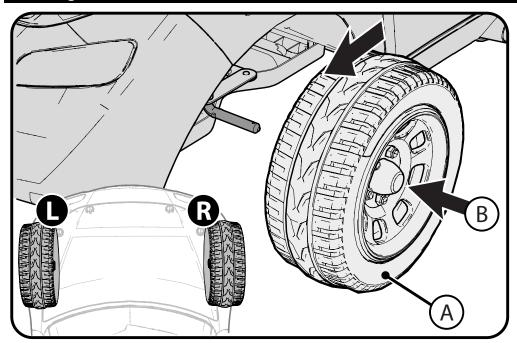
NOTE: Install wheel marked **①** on Left and wheel marked **②** on Right and with center tread pointing FORWARD - looking from the top.
