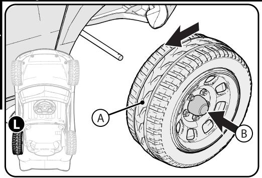
NOTE: Install Wheel marked **()** on Left with center tread pointing FORWARD - looking from the top.
