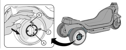
**WARNING:** Hub Lock must be snapped firmly into position to operate correctly.
