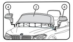
Install the windshield (2) and rearview mirrors (4) by inserting the tabs into the vehicle slots as shown. Press tabs in until a "snap" is heard.
