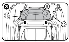
Insert the backrest (8) into place as shown and install the backrest screws (16) securely.
