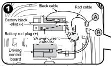
When battery is installed or replaced, insert the Red cable terminal into the Red battery positive pole and the Black terminal into the Black battery negative pole. St. 2 16 16 16
