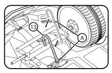
With the vehicle upside down, insert the long end of the J-shaped Steering Rod (13) into the body opening so that short end fits into the axle slot as shown and the fixed washer (A) sits against the car body.
