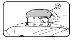
Insert the dashboard accessory (21) into the tab holes until they 'snap' securely.
