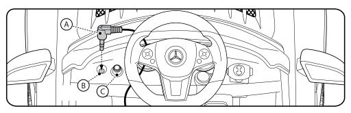
Insert the MP3 Plug (A) into the Socket on the instrument panel (B). Adjust volume by turning the Volume Knob (C) (next to the MP3 Socket).
