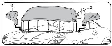
Install the windshield (part 2) and rearview mirrors (part 4) by inserting the tabs into the vehicle slots as shown. Press tabs in until a "snap" is heard.
