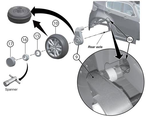
NOTE: Begin by turning the vehicle upside down and removing nuts and washers from axle.
