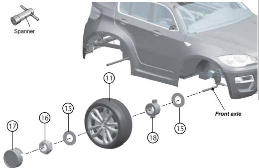
NOTE: Begin by removing nuts and washers from axles.
