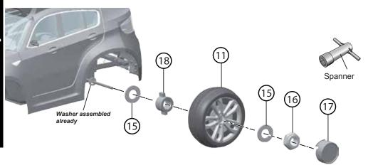
NOTE: With vehicle still upside down, remove nut and washer from axle.
